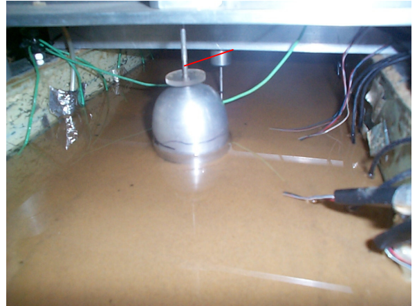
BG-05, approximate tilt angle 6^\circ
