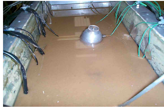
Tilt and rotation of dome after test BG-02
