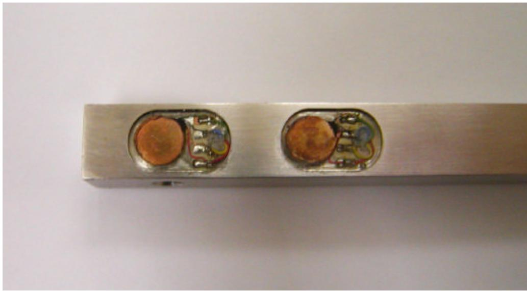
Figure 5. Miniature pressure cells B1 and B2 mounted on pile surface
