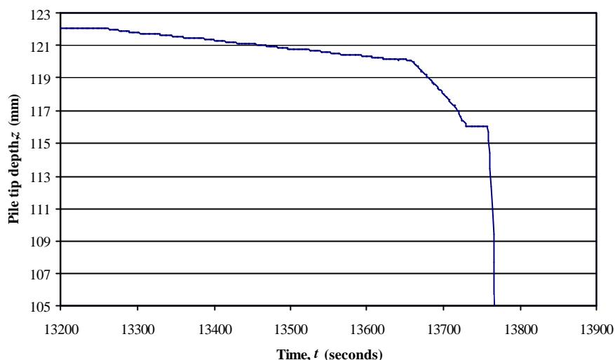
Figure 148 Test T3, Pile tip depth vs. time (load test 4: tension at L)
