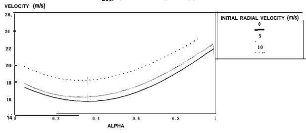
Figure 23a, b & c - Variation of Impact Velocities with Alpha and Initial Radial Velocity for Impact Radius of 260mm
