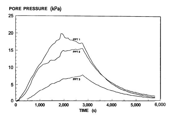
Figure 17e - Test 2. Unreinforced Embankment. Excess Pore Pressures within Clay
