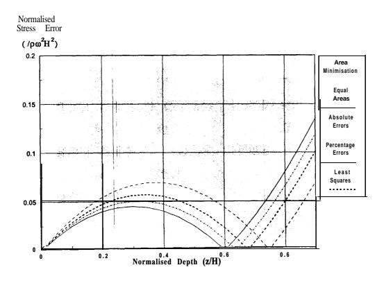
Figure A5b - Normalised Errors vs Normalised Depth - 0.9H as Lower Limit
