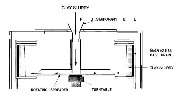
Figure 5 - Clay Pouring Technique
