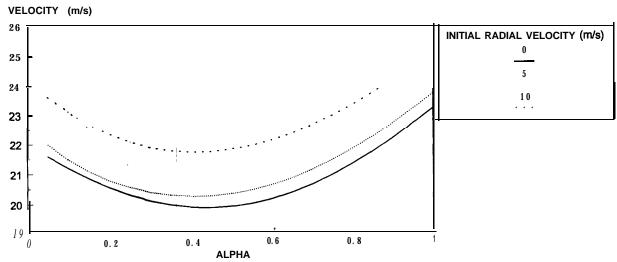
Figure 23d, e & f . Variation of Impact Velocities with Alpha and Initial Radial Velocity for Impact Radius of 320mm
