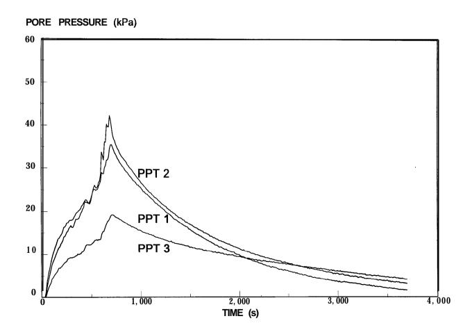
Figure 27b • Test HB04. Unreinforced Embankment. Excess Pore Pressures within Clay
