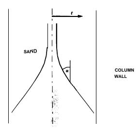
Figure 20 - Sand Profile in Vertical Rotating Column
