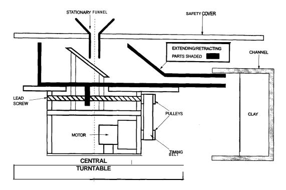
Figure 15d - Schematic Section Through Hopper
