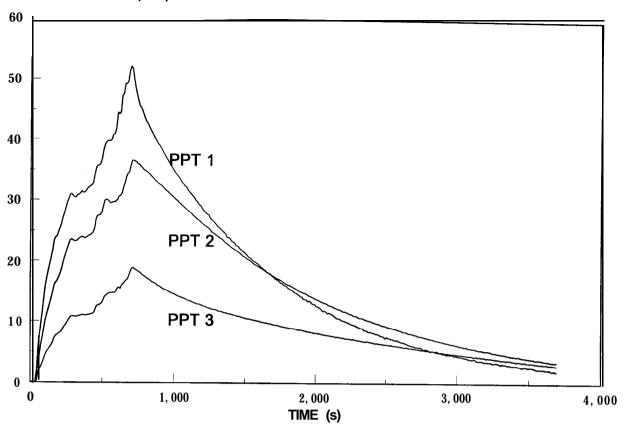
Figure 27a - Test HB04. Reinforced Embankment, Excess Pore Pressures within Clay
