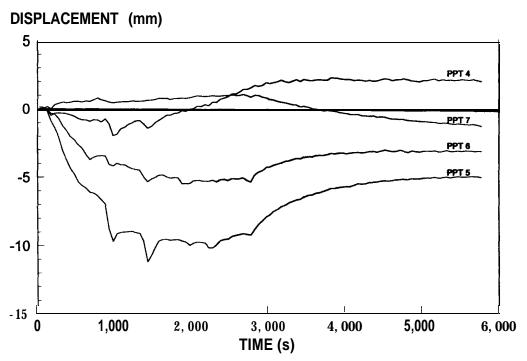
Figure 17g - Test 2. Unreinforced Embankment. Surface Settlements.
