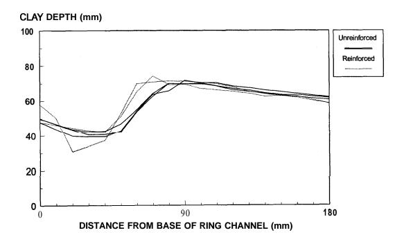
Figure 26 - Post-construction Clay Surface Profiles for Reinforced and Unreinforced Sections.
