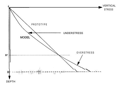
Figure Al • Model Stress Error
