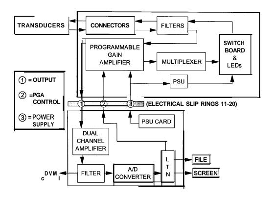
Figure 4 - Schematic Diagram of the Mini-Drum Data Acquisition System
