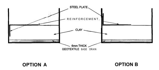
Figure 13 - Reinforcement Plate Orientation Options
