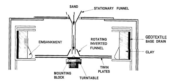
Figure 21 - Section Through Twin Plate Equipment installed in Mini-drum
