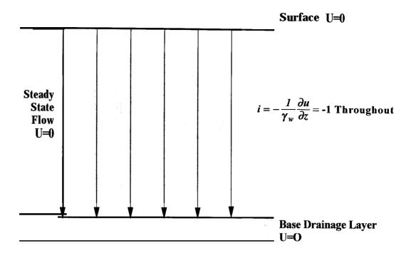
Figure 7 - Steady State Condition, Standpipe Fully Lowered
