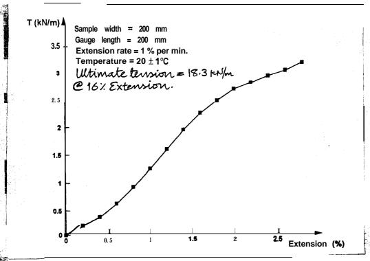
Figure 12 - Load-Extension Curve for Akzo Geotextile Reinforcement (After Sharma (1994))
