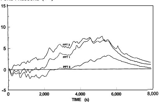
Figure 17b - Test I. Reinforced Embankment. Excess Pore Pressures within Clay
