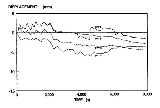
Figure 17d - Test I. Reinforced Embankment. Surface Settlements
