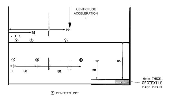
Figure 25 - PPT Locations. Test HB04 (Dimensions in mm)
