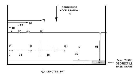
Figure 14 - PPT Locations, MEng Tests (Dimensions in mm)
