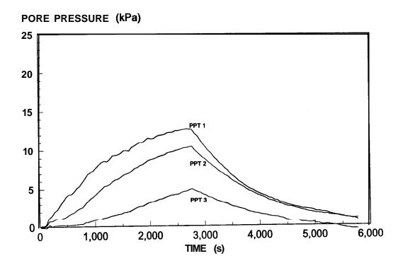
Figure 17f - Test 2. Reinforced Embankment. Excess Pore Pressures within Clay
