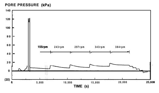
Figure 8 - Test HB01, Day 1. Response of PPT situated 27mm above channel base
