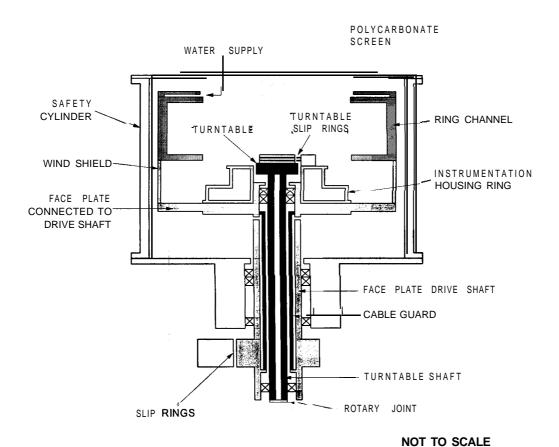
Figure 2 - Section through Mk II Mini-Drum Centrifuge with Axis Vertical
