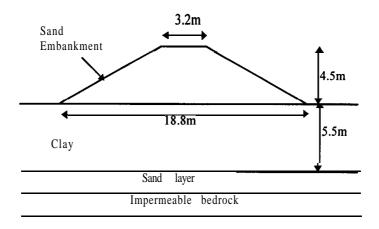
Figure 1. Prototype modelled in centrifuge tests
