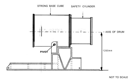
Figure 1 - Elevation of the Mk II Mini-drum Centrifuge with Axis Horizontal
