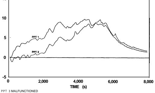
Figure 17a - Test 1. Unreinforced Embankment. Excess Pore Pressures within Clay
