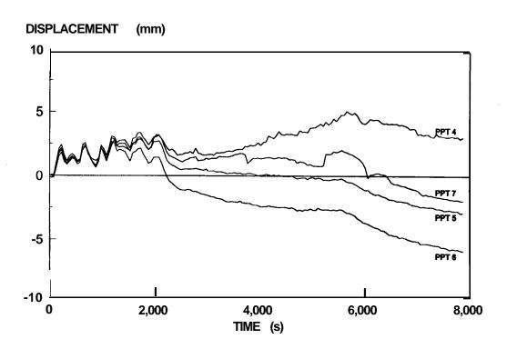
Figure 17c • Test 1. Unreinforced Embankment. Surface Settlements
