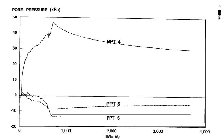
Figure 27c - Test HB04. Reinforced Embankment. Surface Pore Pressure Transducers.
