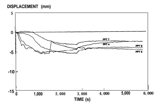
Figure 17h - Test 2. Reinforced Embankment. Surface Settlements.
