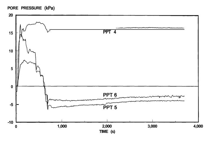
Figure 27d - Test HB04. Unreinforced Embankment. Surface Pore Pressure Transducers.
