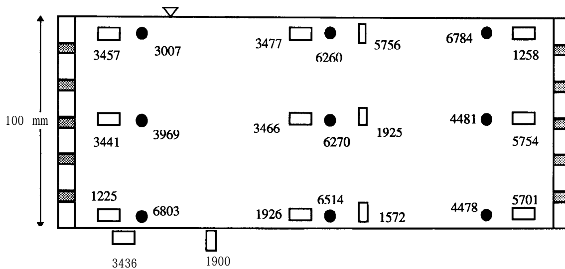
Fig. 32: Schematic diagram showing the placement of transducers in Centrifuge Test MG-5
