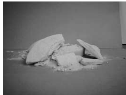
Fig. 10. Blocks of locked sand after oedometer test
