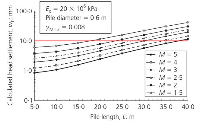
Figure 12. Head settlement ratios for London Clay calculated using Equation 39
