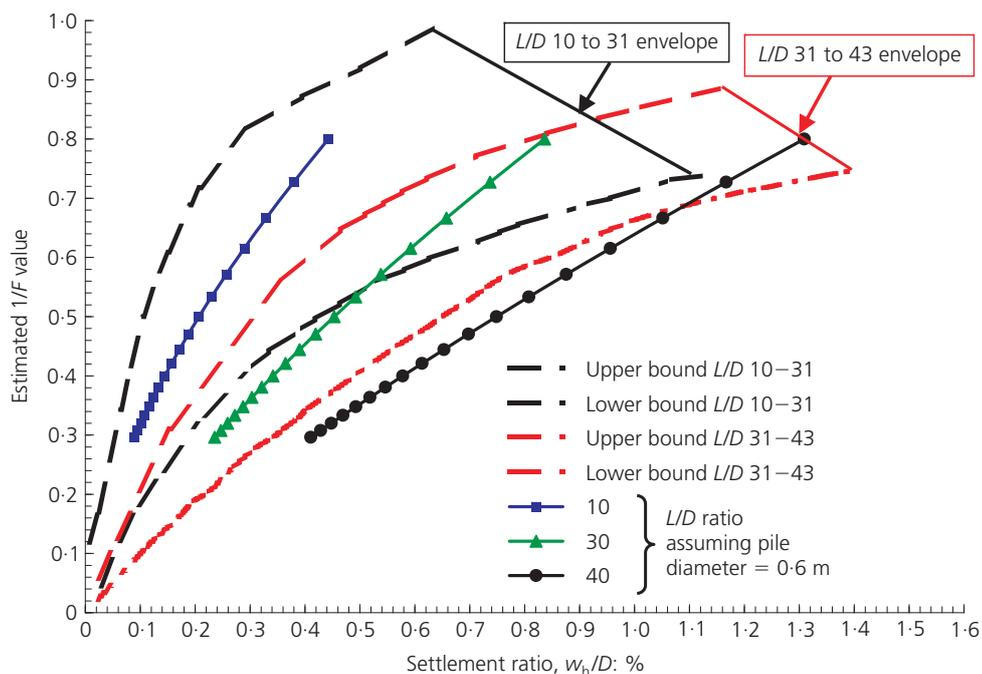
**Figure 14.** Rate-corrected load ratio ( $1/F$ ) plotted against settlement ratio (calculated by Equation 39 for 0.6 m diameter piles;  $c_u = 50 + 7.5z$ )
