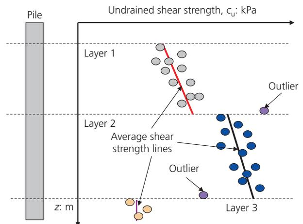
Figure 4. Dealing with soil shear strength variation
