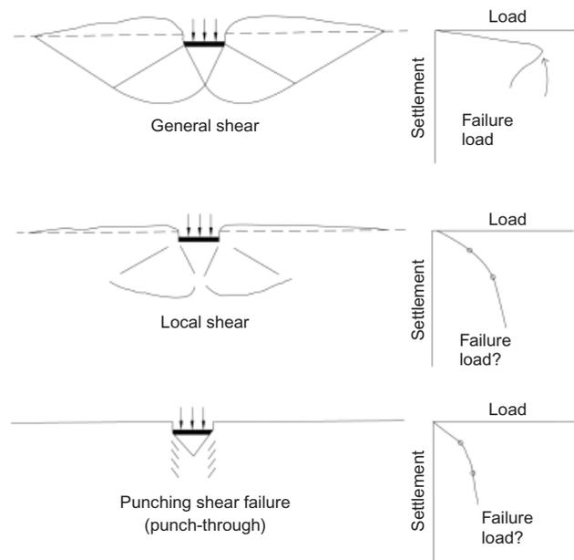
Fig. 1. Modes of failure mechanism (after Vesic, 1963)
