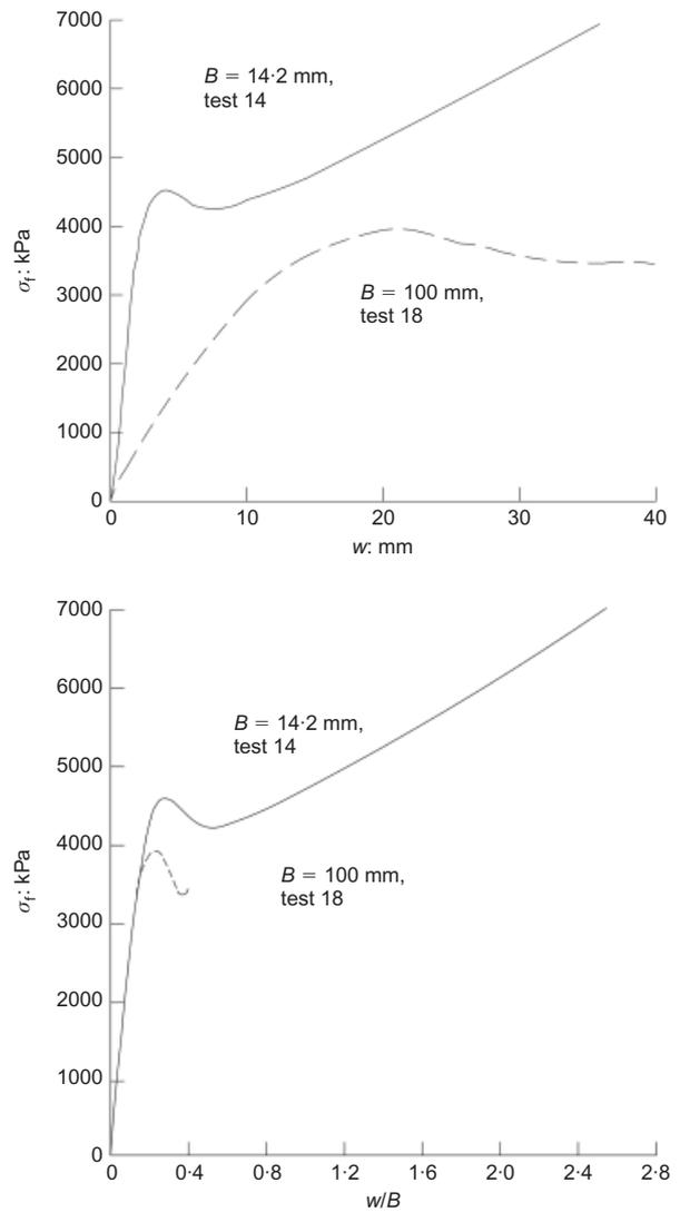
Fig. 9. Comparison between load-settlement response with load-relative settlement response of a footing on sand at  $1g$  with  $\sigma_0 = 10$  kPa
