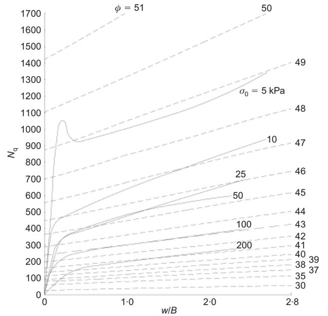
**Fig. 14. Interpretation of 1g test data by superposing the normalised theoretical and experimental curves for silt,  $B = 14.2$  mm**
