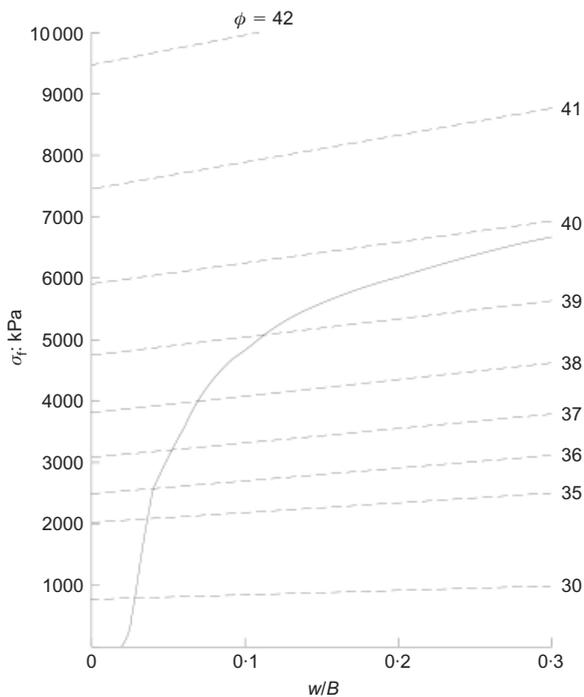
**Fig. 19. Interpretation of centrifuge test data by superposing the theoretical and experimental curves for sand,  $B = 100$  mm at 50g, test 102**
