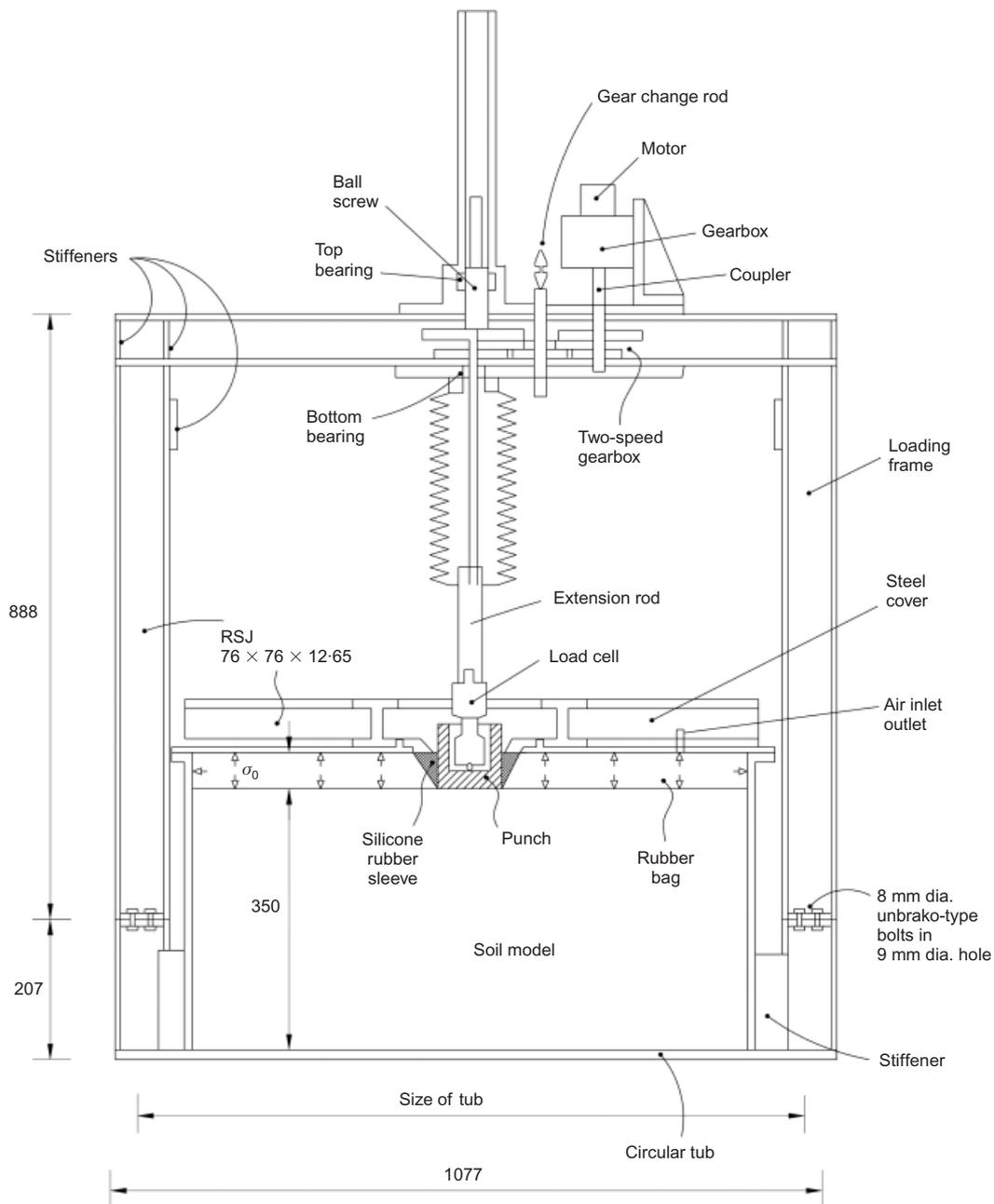
Fig. 8. General layout of test rig at 1g
