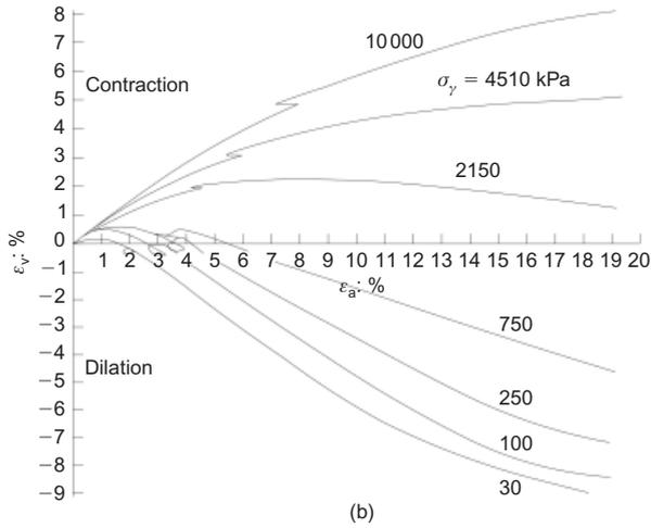
Fig. 4. Effects of effective cell pressure on the stress–strain behaviour of sand in triaxial compression
