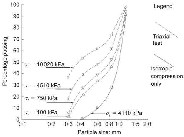
Fig. 7. Grading curves of sand samples after triaxial tests and isotropic compression
