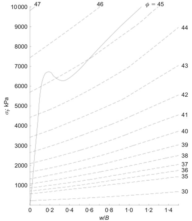
**Fig. 20. Interpretation of centrifuge test data by superposing the theoretical and experimental curves for silt,  $B = 14.2$  mm at 100g, test 104**
