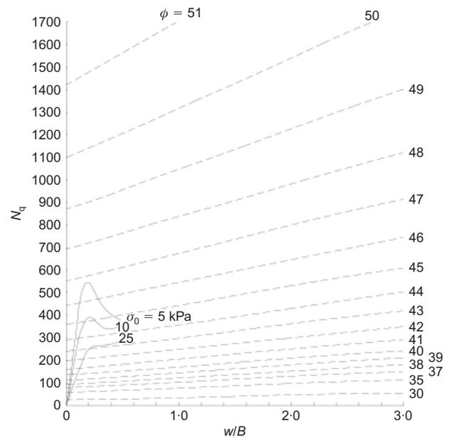
**Fig. 15. Interpretation of 1g test data by superposing the normalised theoretical and experimental curves for sand,  $B = 100$  mm**
