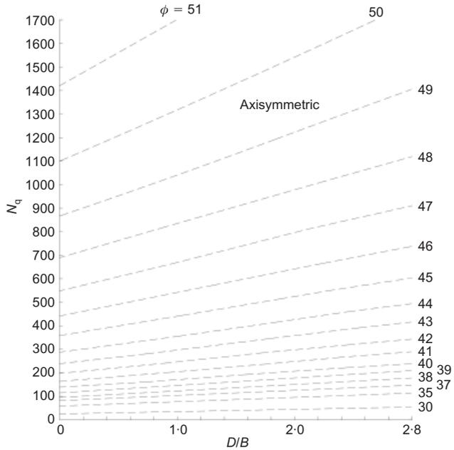
**Fig. 12. Theoretical bearing capacity of shallow footing on weightless soil with overburden with shear strength**
