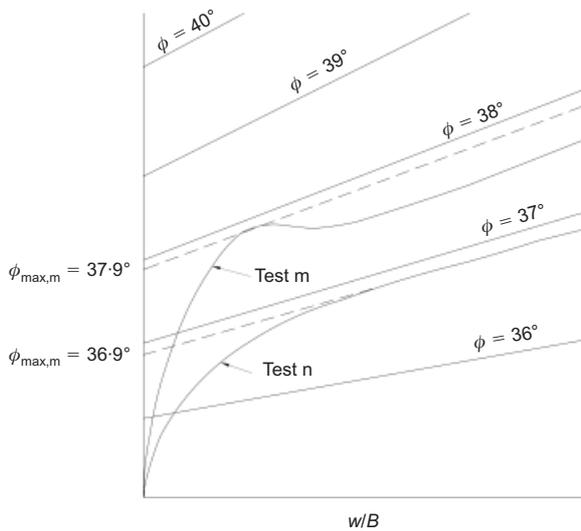
Fig. 16. Schematic diagram showing normalisation of test curves to obtain equivalent  $N_q$  for  $w/B = 0$
