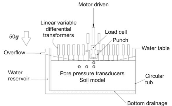
Fig. 18. Model footing apparatus
