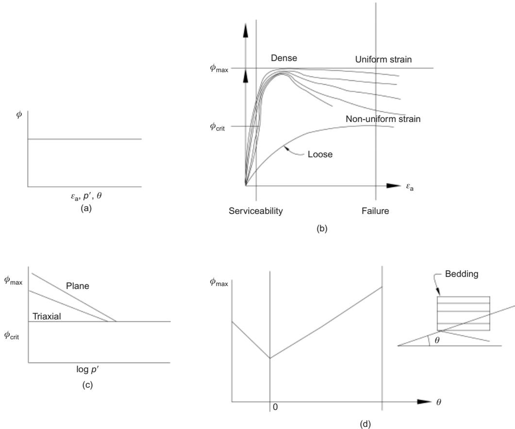
Fig. 2. The variations of  $\phi$  that might concern a practising engineer: (a) ideal soil: bearing capacity equation; (b)  $\phi = f(\epsilon_a)$ ; (c)  $\phi_{max} = f(p')$ ; (d)  $\phi_{max} = f(\theta)$
