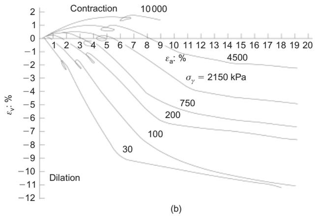
Fig. 5. Effects of effective cell pressure on the stress–strain behaviour of silt in triaxial compression
