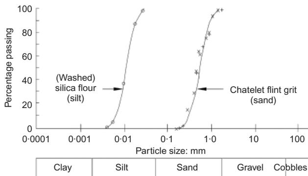
**Fig. 3. Grading curves of the two granular materials**
