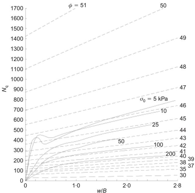
**Fig. 13. Interpretation of 1g test data by superposing the normalised theoretical and experimental curves for sand,  $B = 14.2$  mm**
