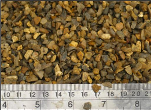
Figure 4. Gravel used as rock-dump
