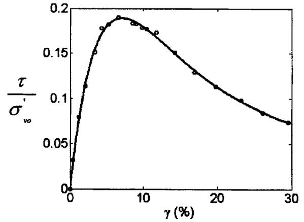
**Fig. 17.** Stress-strain response from an undrained DSS test on Norwegian quick clay [Bjerrum and Landva (1966); reproduced with permission from the Institution of Civil Engineers, London, U.K.]
