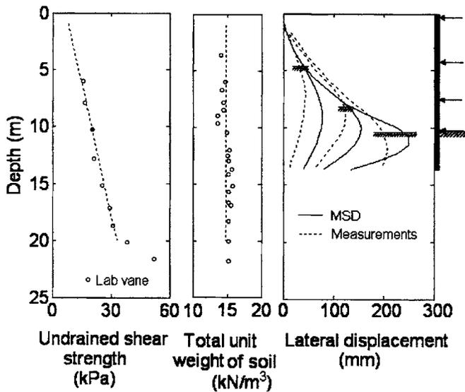
**Fig. 16.** Davidson Avenue: Soil properties and lateral displacements [measurements from Clough and Reed (1984)]
