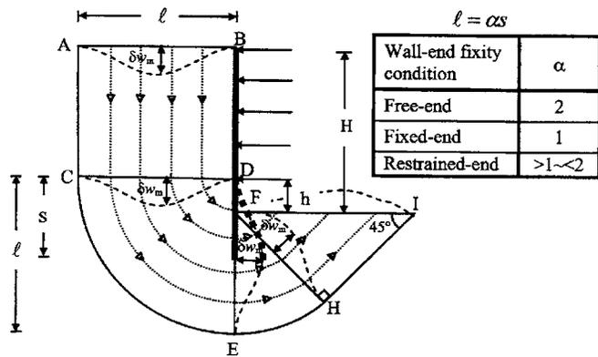
Fig. 3. Plastic deformation mechanisms for braced excavations in clay
