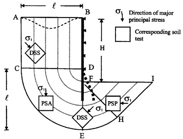
DSS: Direct Simple Shear; PSA: Plane Strain Active; PSP: Plane Strain Passive
