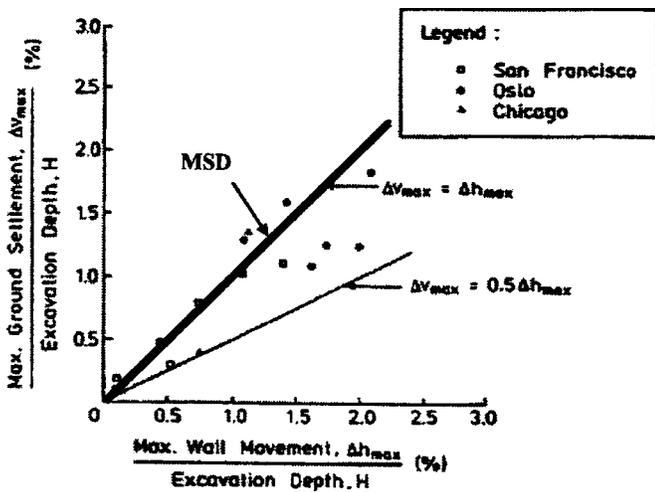
Fig. 8. Relationship between maximum ground settlements and maximum lateral wall movements [adapted from Mana and Clough (1981), ASCE]
