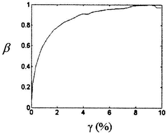
**Fig. 15.** Normalized stress-strain response from a  $K_0$ -consolidated undrained DSS test on Young Bay mud at Islais Creek [data adapted from Hunt et al. (2002)]
