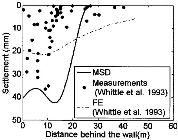
**Fig. 14.** Comparison of predicted and measured surface settlements after the installation of the sixth floor at Boston Post Office Square Garage
