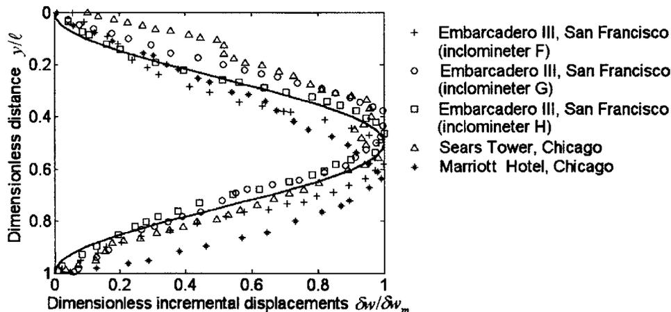
Fig. 2. Comparison of incremental displacement profiles between field inclinometer data and the cosine function [data adapted from O'Rourke (1993); with permission from the Institution of Civil Engineers]
