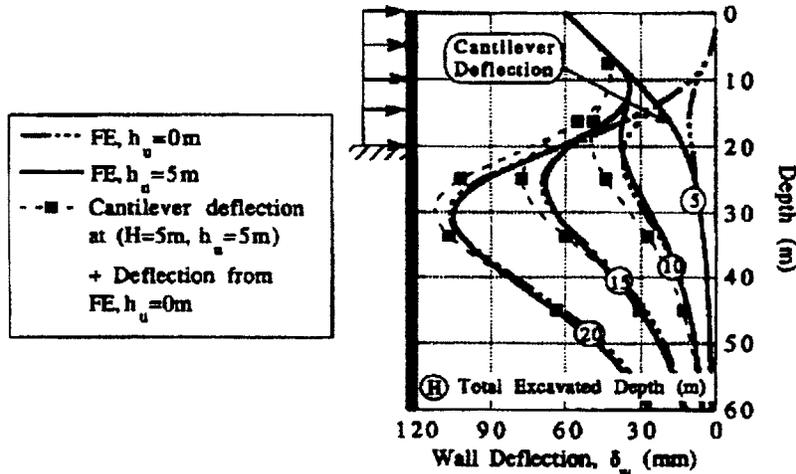
**Fig. 6.** Comparison between FE analysis and the Clough et al. (1989) method for the effects of cantilever stage movements on system displacement [Hashash (1992); reproduced with permission from MIT]
