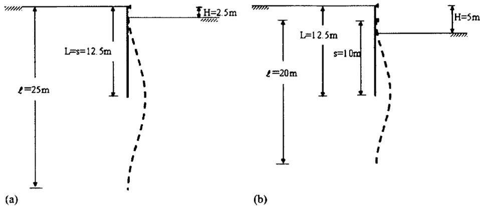
Fig. 19. Bulging incremental movement: (a) Step 2 and (b) Step 3
