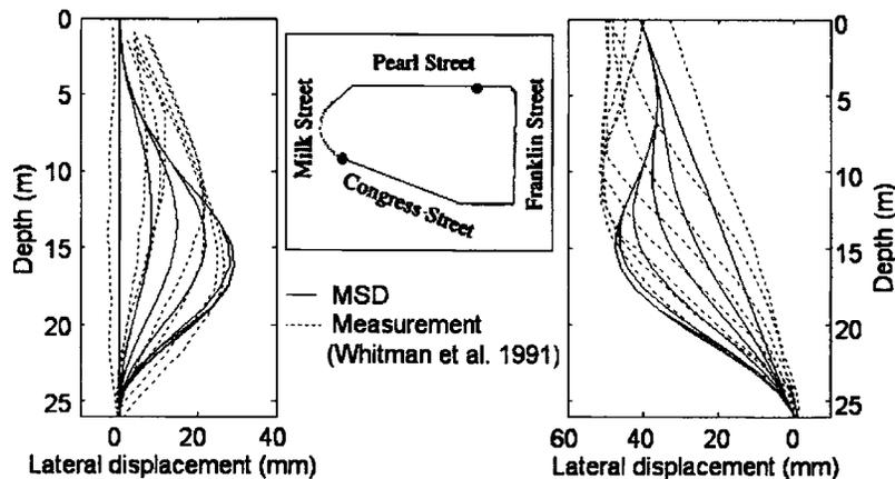
Fig. 13. Predicted and measured lateral displacements at Post Office Square Garage
