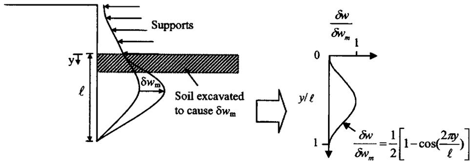
Fig. 1. Incremental displacements in braced excavations [adapted from O'Rourke (1993)]
