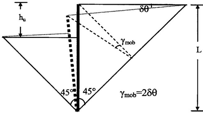
Fig. 7. Plastic deformation mechanism for cantilever retaining walls in undrained conditions
