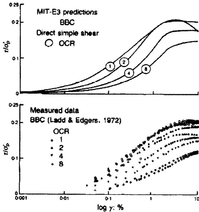
Fig. 10. Stress-strain response for  $K_0$  consolidated undrained DSS tests on Boston blue clay [Whittle (1993); reproduced with permission from the Institution of Civil Engineers, London, U.K.]
