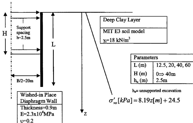
Fig. 9. Initial conditions and geometric parameters [adapted from Hashash and Whittle (1996)]
