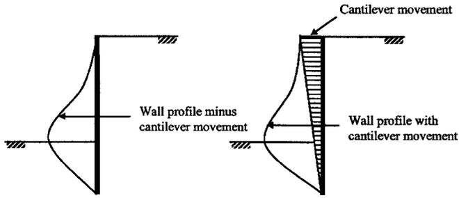
**Fig. 5.** Effect of cantilever stage movements on system displacement [adapted from Clough et al. (1989)]
