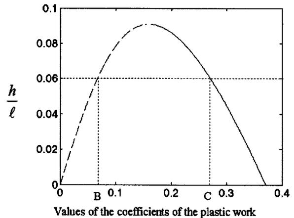
Fig. 20. Values of coefficients of the plastic work in the distributed shearing zone EFH (coefficients B and C of Table 3)
