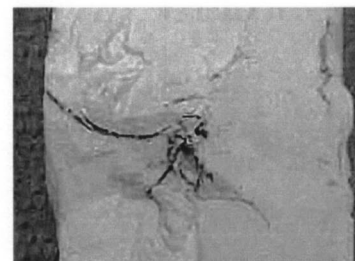
(c) Cement bentonite ( w/c=3 ) in OCR = 1 specimen
