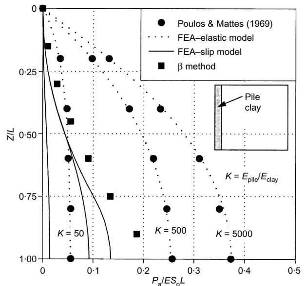
Fig. 3. Distribution of dragload as determined by various methods.  $E_{pile} = 2 \text{ GPa}$ ,  $\Delta p = 25 \text{ kPa}$ ,  $\mu = 0.3$ ,  $\beta = 0.3$
