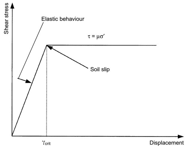
Fig. 2. Behaviour of interface element
