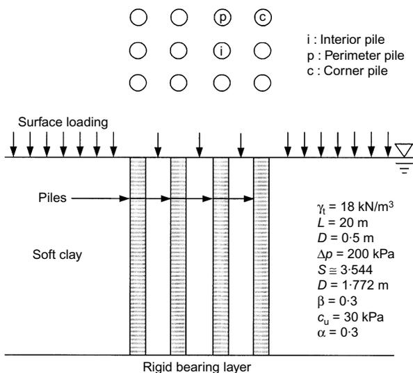
Fig. 14. Configuration of a pile group by Combarieu (1985)
