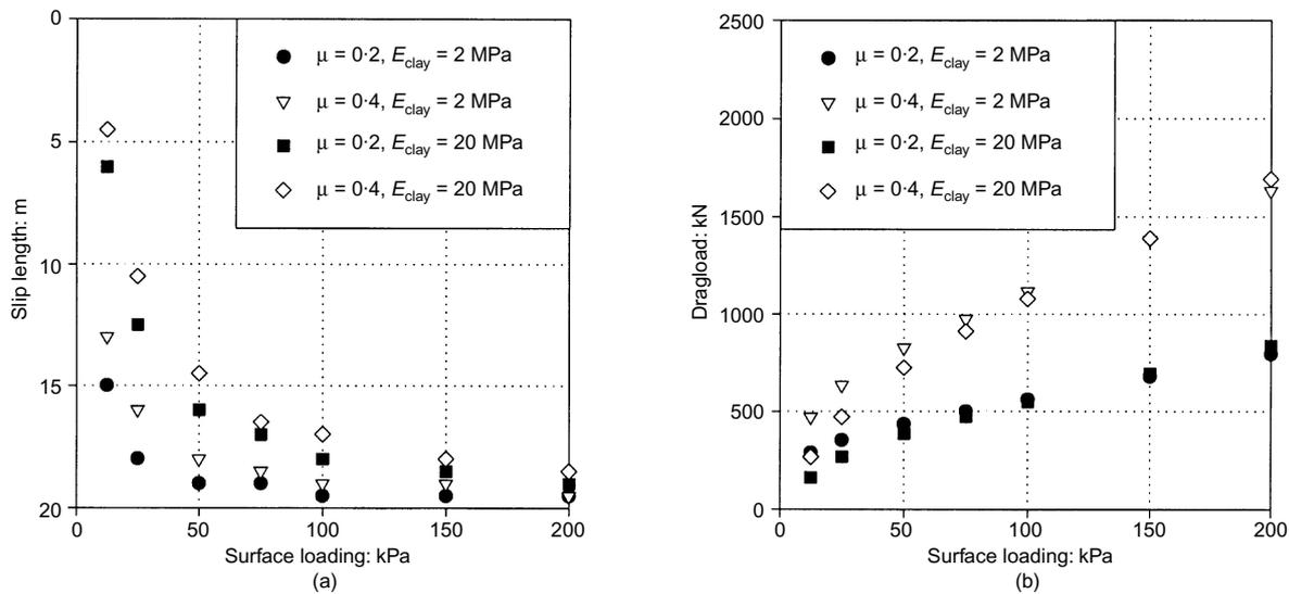
Fig. 5. Effect of soil slip at the interface: (a) slip length; (b) dragload
