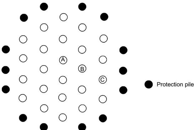
Fig. 11. Configuration of group of 38 piles (Okabe, 1977)
