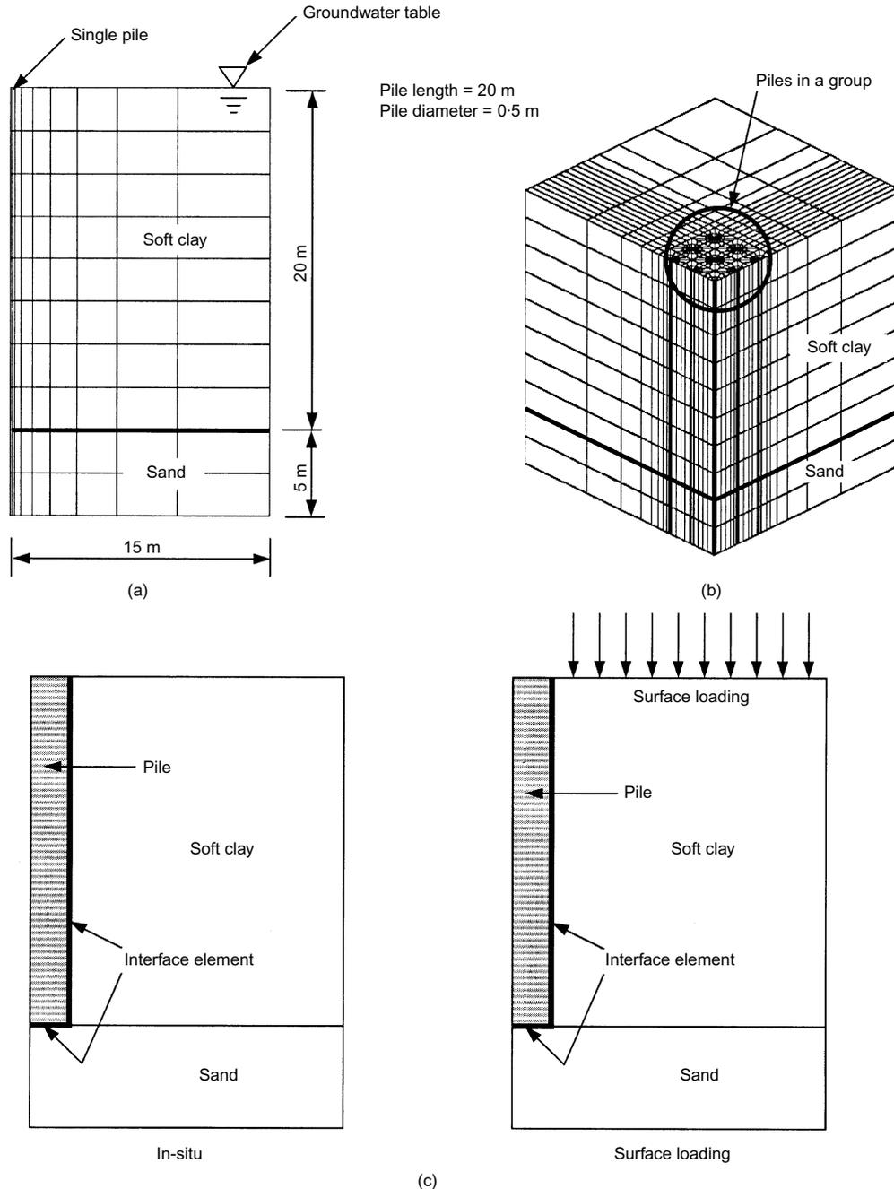
Fig. 1. Typical FE meshes for (a) 2D (axisymmetric) and (b) 3D (5x5 piles in 2.5D) analyses; (c) analysis sequences
