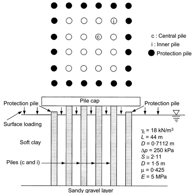
Fig. 12. Configuration of pile group simulated in FEA to model full-scale experiment by Okabe (1977)
