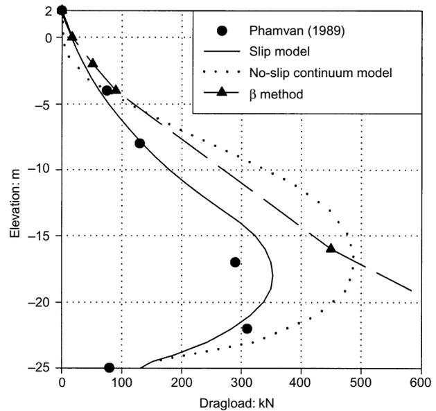
Fig. 9. Comparisons of the development of dragload
