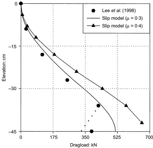
Fig. 10. Fitting the slip model to centrifuge data
