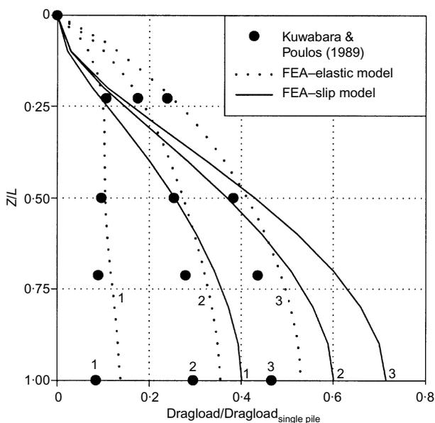
Fig. 6. Comparison of dragload with and without slip.  $S = 5.0D$ ,  $E_{clay} = 20 \text{ MPa}$ ,  $\Delta p = 25 \text{ kPa}$ ,  $\mu = 0.3$ . See Fig. 7(a) for position of the piles
