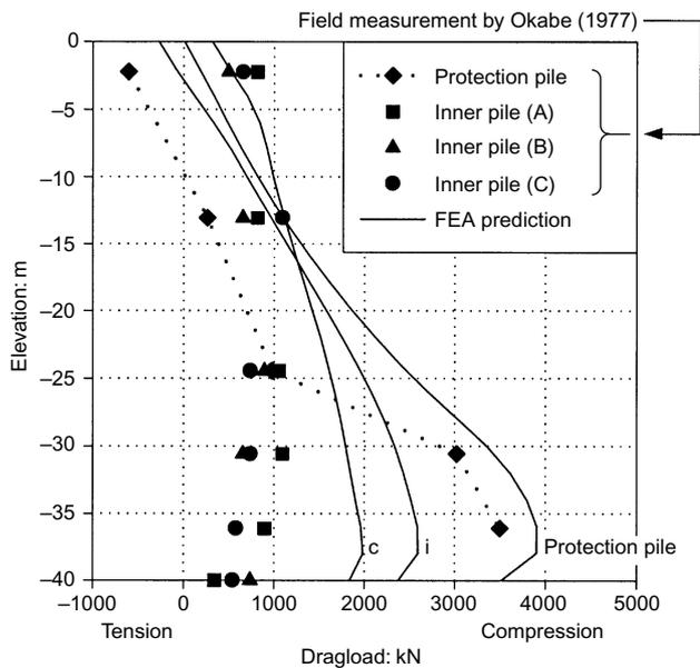
Fig. 13. Distribution of dragload (see Figs 11 and 12 for positions of the piles)
