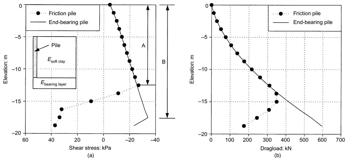
Fig. 4. (a) Shear stress and (b) dragload distributions.  $E_{\text{soft clay}} = 5 \text{ MPa}$ ,  $\mu = 0.3$ ,  $\Delta p = 50 \text{ kPa}$ .  $E_{\text{bearing layer}} = 5 \text{ MPa}$  (friction pile), 5 GPa (end-bearing pile). A, slip length for a friction pile; B, slip length for an end-bearing pile
