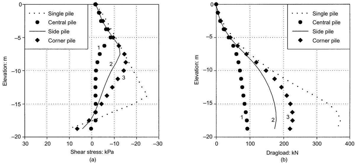
Fig. 8. Development of group effect (see Fig. 7(a)): (a) shear stress; (b) dragload.  $S = 2.5D$ ,  $E_{clay} = 5 \text{ MPa}$ ,  $\mu = 0.3$ ,  $\Delta p = 25 \text{ kPa}$
