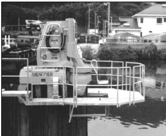
Figure 1; Silent piler with safety walkway
