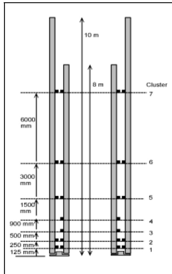
Figure 5; Strain gauge locations
