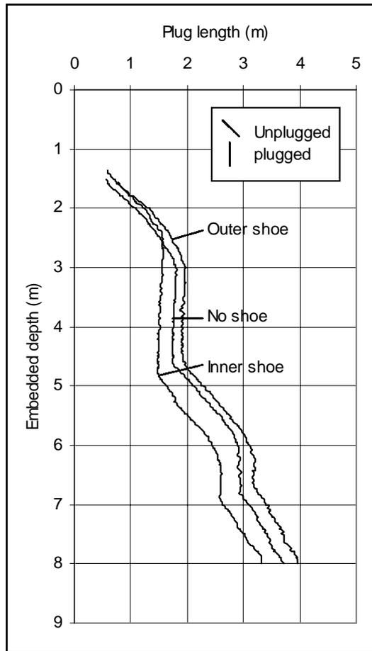
**Figure 7; Plug length vs Embedded depth**
