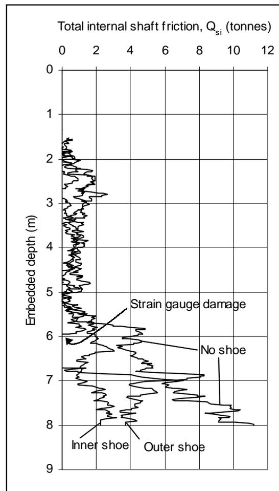
**Figure 12; Total internal shaft friction vs embedded depth**
