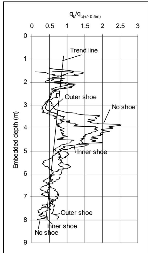
**Figure 10; Normalised unit base resistance ( $q_b/q_{c(+/-0.5m)}$ ) vs Embedded depth**
