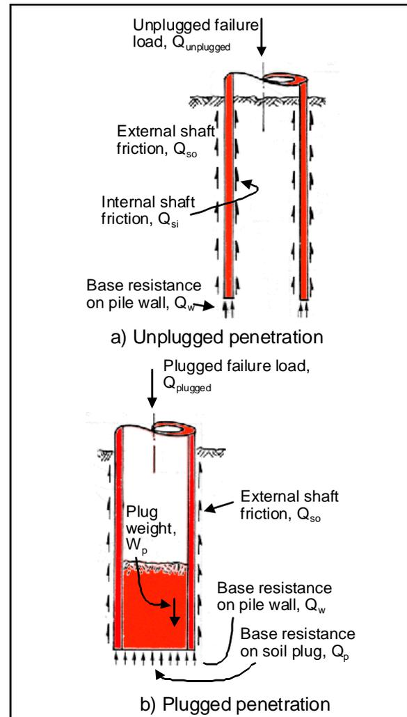
**Figure 8; Plugged and unplugged modes of penetration**
