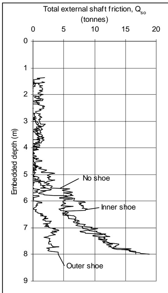
**Figure 11; Total external shaft friction vs embedded depth**
