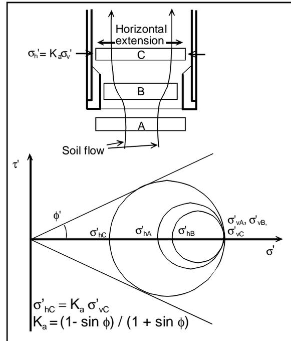
Figure 2; Hypothesised stress changes around a driving shoe [3]
