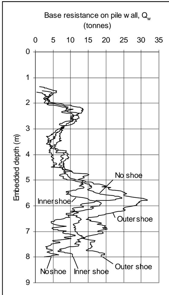
**Figure 9; Base resistance on pile wall,  $Q_w$  vs Embedded depth**
