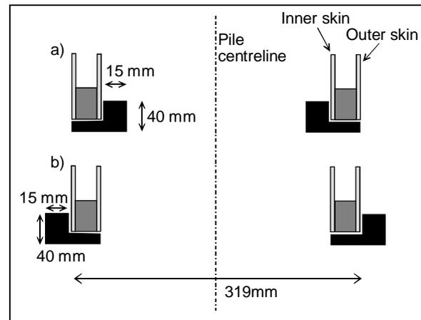
Figure 4; Driving shoe dimensions
