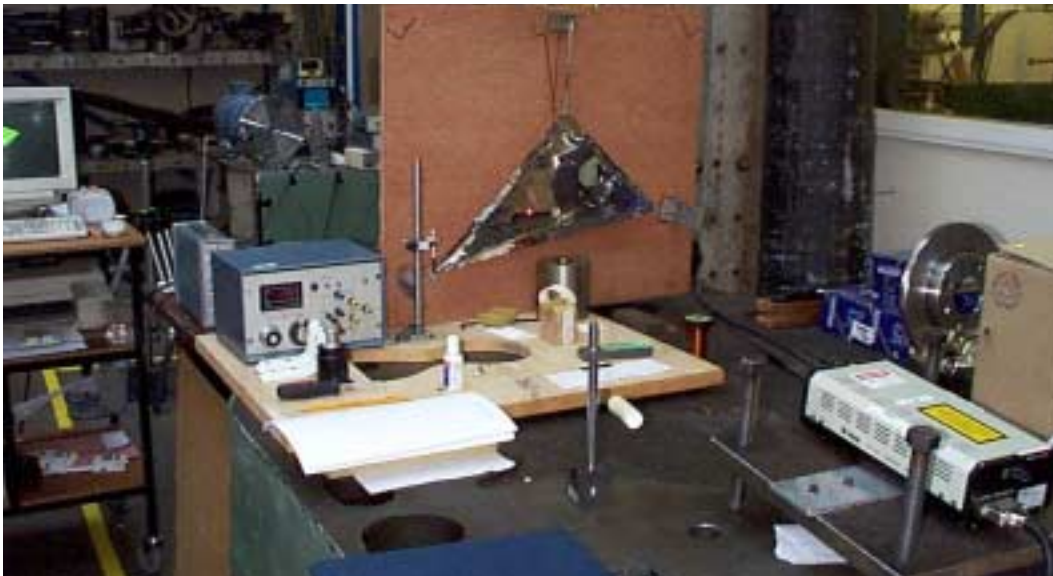
Figure 5.3: Experiment set-up for impulse excitation.
