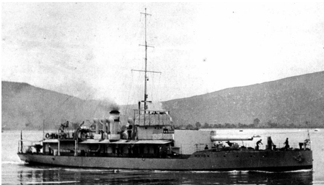
M18 at Stavros. The hull was clearly built around the gun she was to carry. (IWM)
