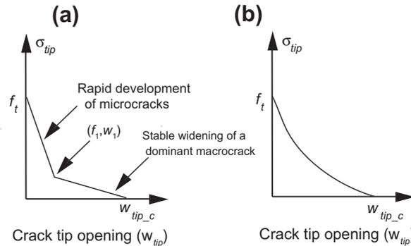
Fig. 8. Simplified tension-softening models (a) bilinear and (b) polynomial.
