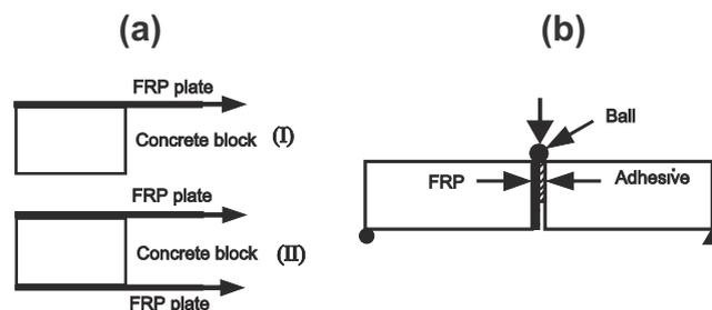
Fig. 5. (a) (I) – single (II) – double shear lap specimens. (b) A three-point bend specimen.
