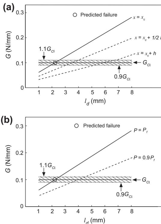
Fig. 12.  $G$  vs.  $l_d$  plot for Group 1 beam (Ross et al. [33]) for fractures starting at (a) different locations and (b) 90% of the failure load.
