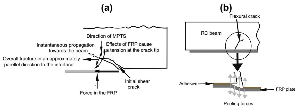
Fig. 3. (a) Effect of the FRP causes a significant tension at the tip of the shear crack during PE debonding. (b) Relative sliding between the two faces of flexural cracks causes interface flaws that trigger IC debonding.
