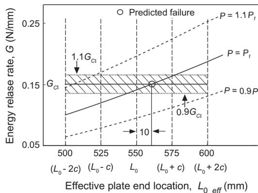
Fig. 10.  $G$  vs.  $L_{0,eff}$  plots for beam set F9 and F10 (Fanning and Kelly [29]).
