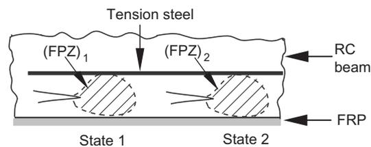
Fig. 6. Crack before and after extension.
