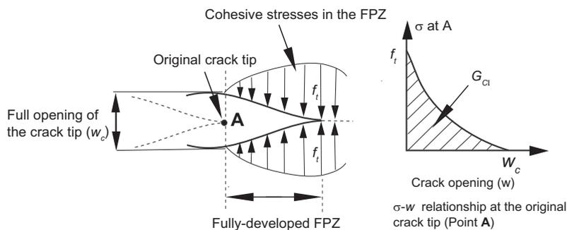
Fig. 7. Cohesive crack model (Hillerborg et al. [21]).
