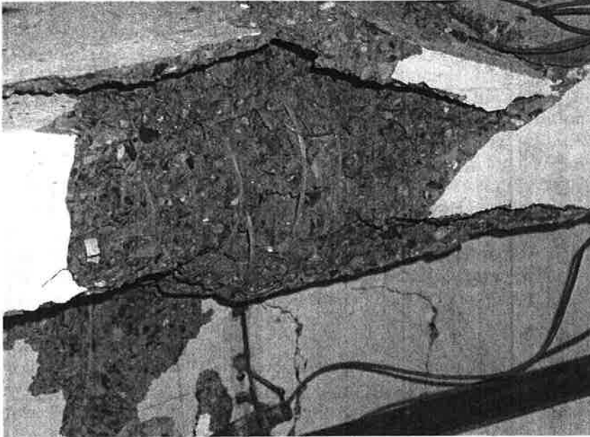
Figure 7—Top flange after spiral snapping
