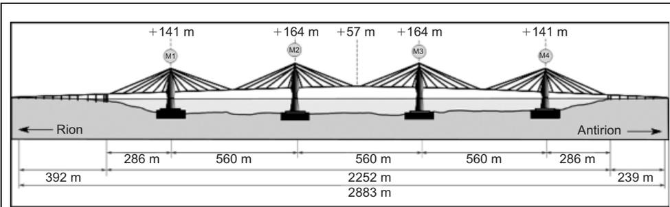
Figure 13. Elevation chart of the Rio-Antirion Bridge
