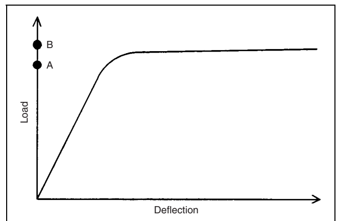
Fig. 9. Load-deflection behaviour of an 'under-reinforced' section
