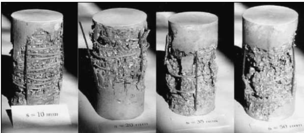
Fig. 11. Compression samples with confinement reinforcement. The samples on the left have more confinement
