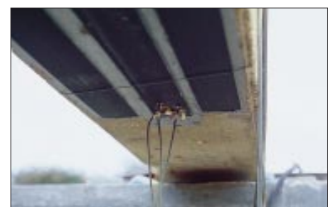
Fig. 1: Bonded plates on test beams
