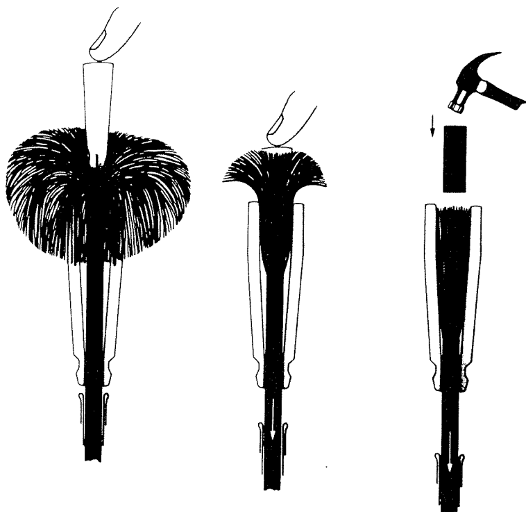
Figure 1. Barrel and spike termination for Parafil.
