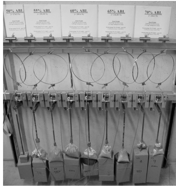
Figure 2 Experimental set-up for CCT tests
