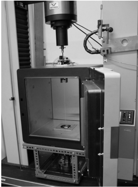
Figure 1 Experimental set-up for tensile and SIM tests
