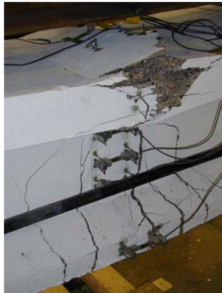
Figure 6. Concrete section at ultimate load (1)
