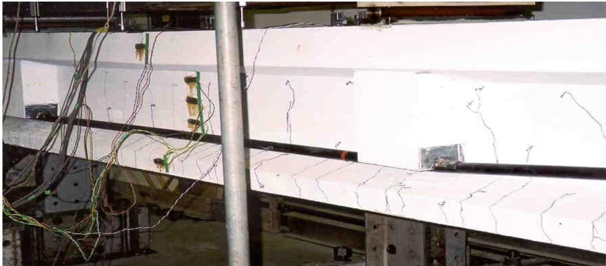
Figure 4. Prestressed concrete beam at 200 kN
