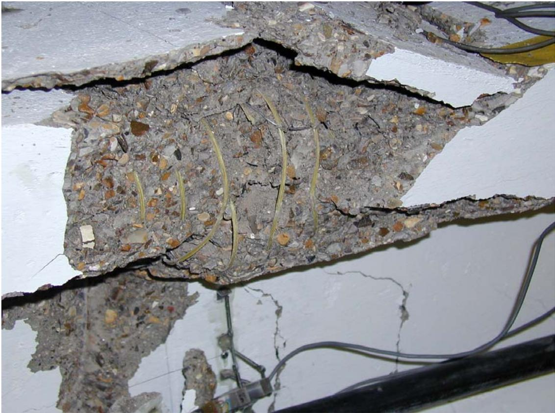
Figure 7. Top flange after spiral snapping
