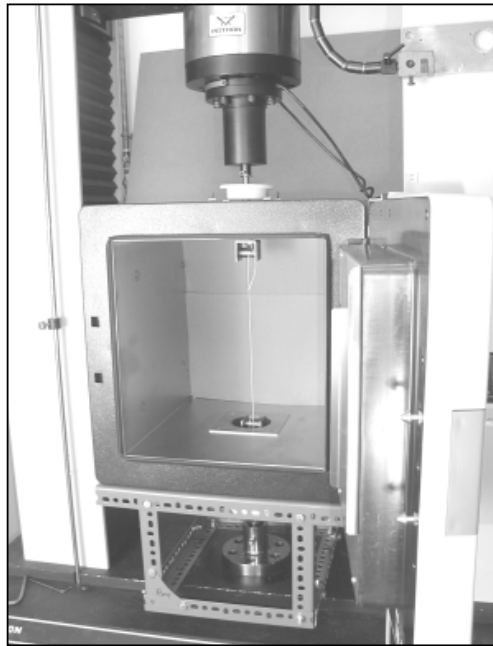
Fig. 2 – Experimental set-up for Tensile, TTSP and SIM test
