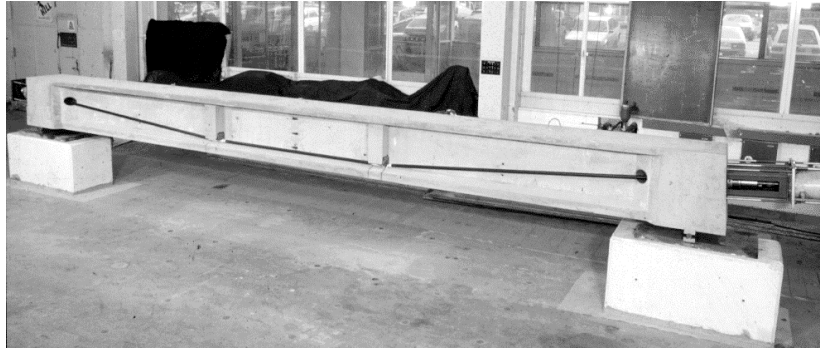
Figure 8 Test beam with external aramid cables
